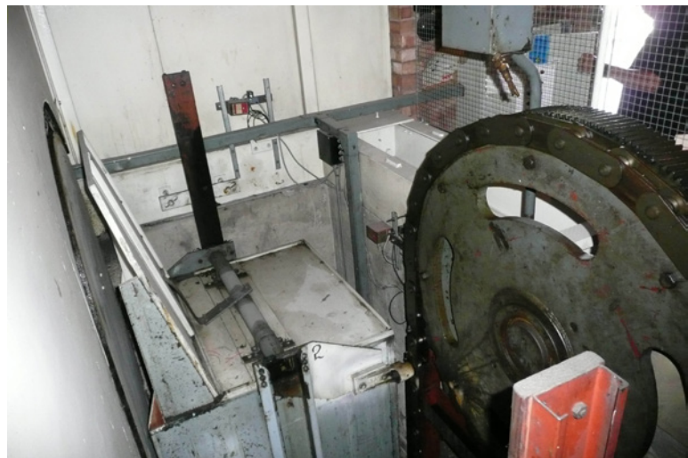
2013,7 and 8. Views showing compartment no. 2 in the position in which it is about to be transferred from one shaft to the other. Images courtesy of M&S. GHJ.
